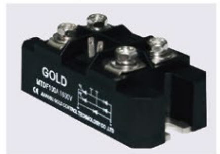
100A单相可控整流桥模块 100A Single-phase Controllable Rectifier Module 型号Type: MTDF-100A 输出耐压VRRM: 1600V 最大输出Max Load Current: 100A 外形尺寸Dimensions: 80 × 40 × 27mm 安装尺寸Fixing size: 67mm, φ 6.5mm
